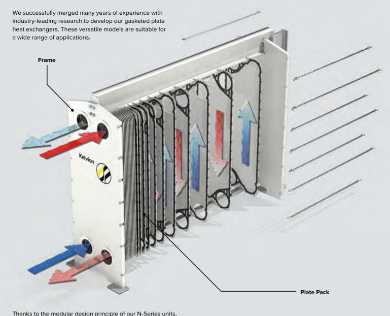
our Sales & Application engineers can choose the most suitable plate series, as well as frame independently, and combine these to find the best configuration of your heat exchanger.
