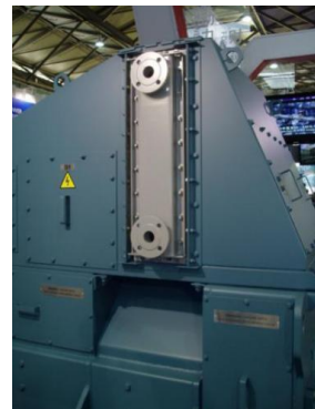
背包式电机空冷器 Package design of air cooler with housing
